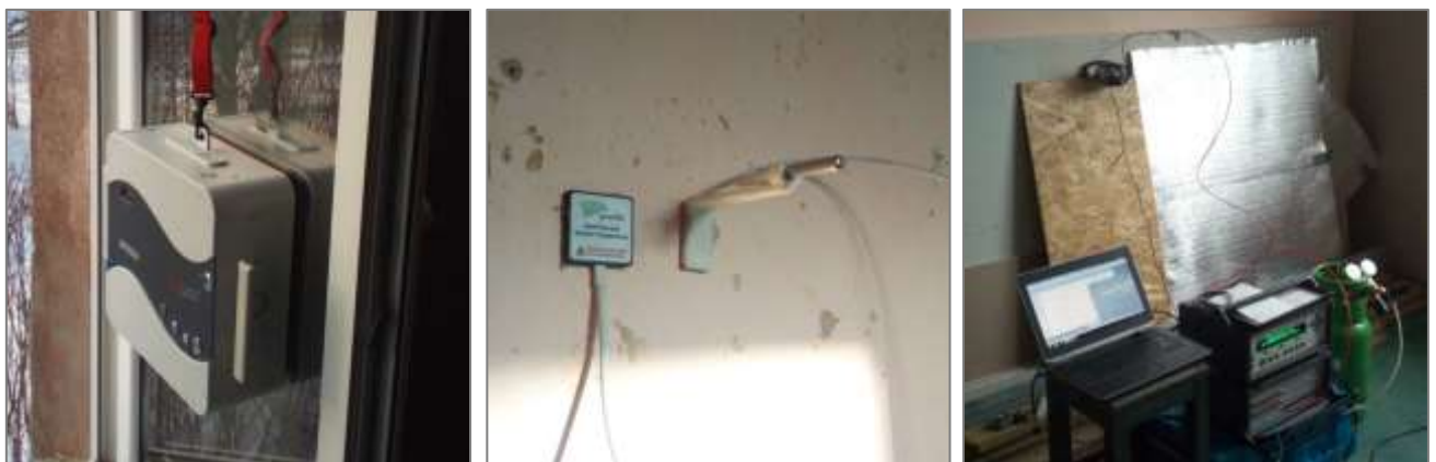
Figure 5. Measurements of thermal transmittance and air change rate.
