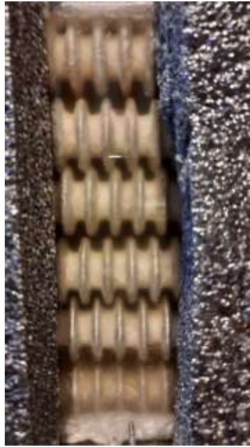
Figure 4. A photo of a heat exchanger with the shape of solidification front after 14 minutes from the beginning of discharging; water flow rate 1.0 l/min, water inlet temperature 45 °C.
