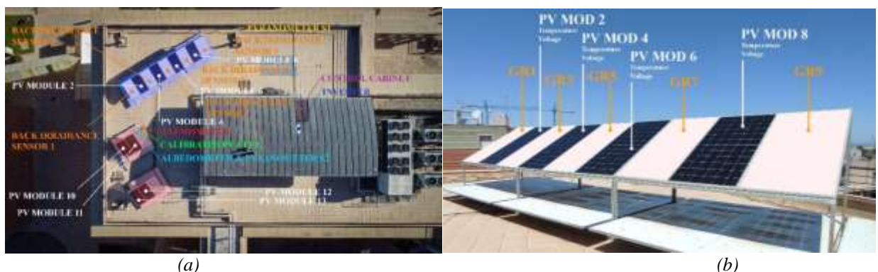
Figure 1. (a) Aerial view of the monitoring system with the elements highlighted. Shaded in blue the modules belonging to string 1 and in red the modules belonging to string 2. (b) Detailed view of string 1. The modules acting as rear irradiance sensors labelled as GR_i , with i=1,3,5,7,9 as well as the generation modules labelled as PV MOD_j , with j=2,4,6,8 are shown in the picture.
