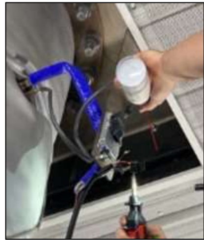
Figure 2. NOx Sensor install detail
