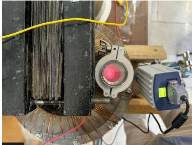
Figure 5. Gas glow in TOKAMAK device
